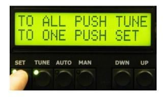
In the case of resetting a single parameter use UP / DWN to select which option and confirm by SET.
