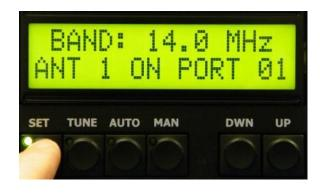
By scrolling UP / DWN you assign which PORT is used on your external antennas switch for this particular antenna. (ANT 1 ON PORT 01).
