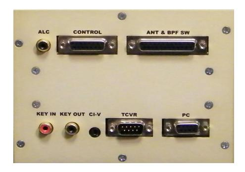
**KEY IN** RCA Phono - Input signal PTT switching voltage / current 5V /2 mA)
