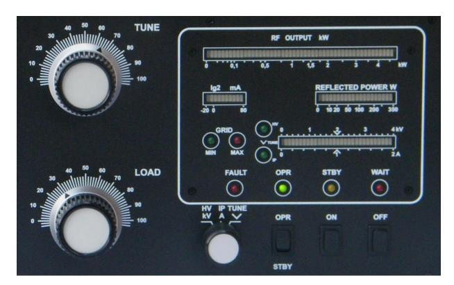
**TUNE** Anode capacitor for tuning, tuning of higher frequencies to "0", lower
