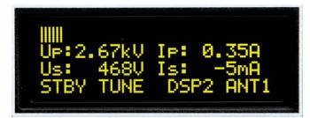
Screen current -5mA is inside the possible working range (from -30mA to +50mA).
