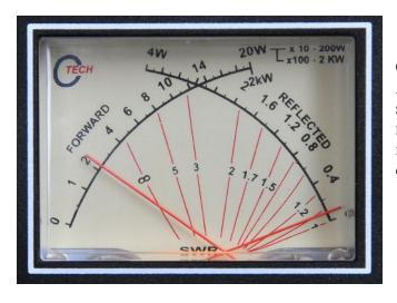
Output power and SWR is visible on the Analog wattmeter, too. This double system meter helps quickly and clearly reaches maximum output power and minimum SWR using both tuning capacitors (TUNE and LOAD)
