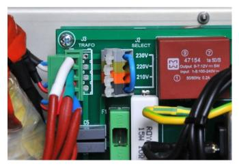
If necessary, manufacturer can prepare selector for other AC range. Here, for example, AC selector was made for the range of 210-230 VAC.
