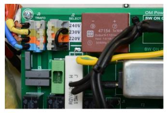
Latest the manufacturer changed the type of connectors for transformer termination. New WAGO connectors they have different colour for every contact. This corresponds approx. to the shrink foil colour of transformer terminals (white, yellow, orrange, blue - primary wiring - J3 connector).
