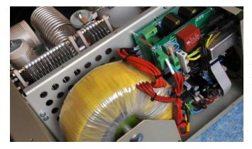
Power amplifier is using a 2.3 kVA toroidal transformer. A soft start is provided using relays and resistors (on the front board).
