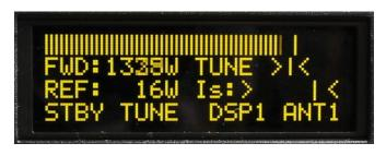
Display indicates the **correct tuning** of the Power amplifier.
