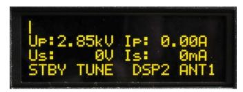
Without RF power the plate voltage is 2.85 kV. It is not good enough.
