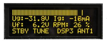
...and the heating voltage drops to 6.2V.
