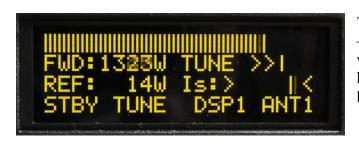
Two of important information is visible – screen current increased, but still is within the allowed limits. Turn LOAD knob slightly to get TUNE indicator between arrows.
