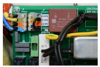
Use flat screwdriver or finger and press carefully the white stick to release contact and move upper end of the black jumper to the proper position, if necessary.
