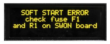
If resistor R1 or fuse F1 is damaged, safety circuit stops starting of the PA and fault message appears on the display. If this occurs, contact your dealer, please.
