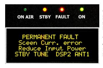
This is the situation, when problem with high Input power persists. Safety circuits reacted 3 times, and then switched PA to STBY mode. Permanent fault appears.
