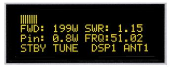
Then we applied input power from handy TCVR. Basic parameters are visible on the display.
