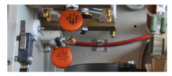
One special fuse is used in the model OM1500. In the case of an accidental discharges in the tube this fuse saves HV supply circuits.
