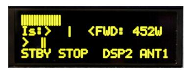
Effect of included input attenuator is visible; power output is low. TUNE position (third row) is not a good. Use **LOAD** knob to move it to the center.
