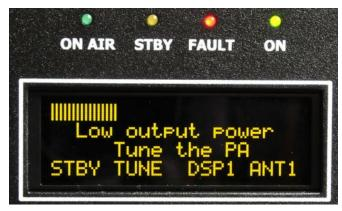
Safety circuit stopped transmitting, fault LED is **ON** (Fault code 4 is saving to the memory).
