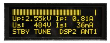
During transmitting the plate voltage drops to 2.55 kV,
