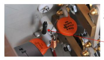
Fuse is installed behind TUNE capacitor, close to the blower.
