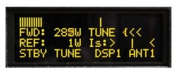
This is not an optimal result, TUNE indicator must go between both arrows. Use TUNE knob to get maximum output power and LOAD knob to get indicator between arrows.
