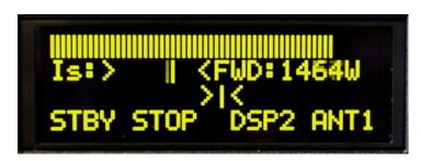
Display shows properly tuned PA. TUNE indicator is in the middle, Screen current is higher, but still inside the limits.
