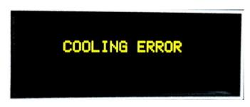
Another example shows situation, when blower stops running. Safety circuits immediately switch PA OFF. Fault message stays on the display only.
